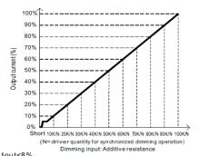
Note: 1. Min. dimming level is about 8% and the output current is not defined when 0% < Iout < 8%.
