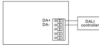
Note : Maximum DALI cable length is 300m (based on a 1.5mm<sup>2</sup> or 14AWG cable)
