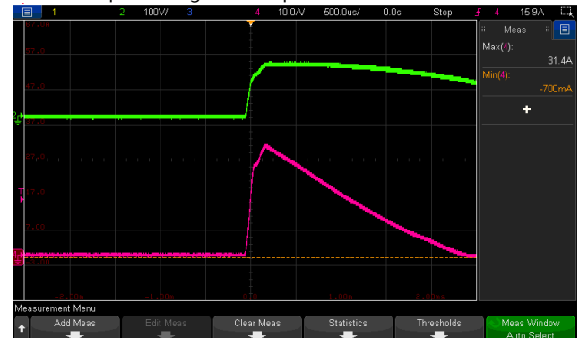
INPUT=115VAC/60HZ @ FULL LOAD CH2: AC Input Voltage CH4: Input current
