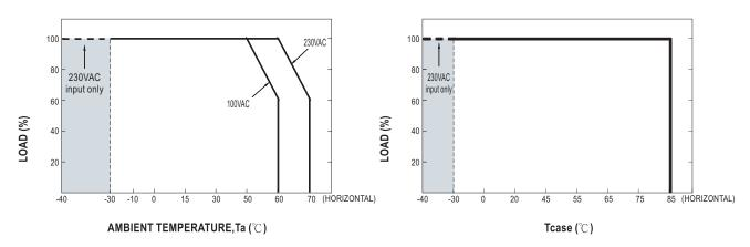
Note:1. The output current must be derated at ultra-high ambient temperature. 2.Below 120VAC@-30°C may has restart situation within 5s after power-on.
